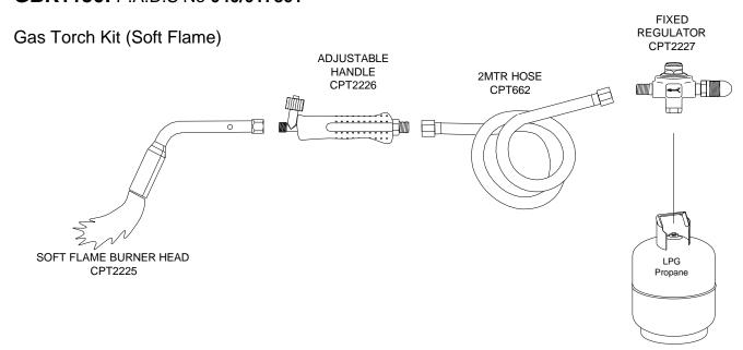
This gas torch delivers a soft flame from standard LPG/BPG gas bottles. It is ideal for use with Low and high Voltage Heatshrinkable jointing systems. The kit comprises of a soft flame burner head, an adjustable handle, 2 metre hose and regulator.
