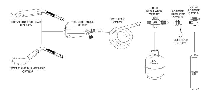
This Gas torch kit is designed for heatshrink jointing and can be used with Primus 2000 or standard LPG/BPG refillable steel containers.
