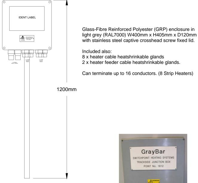
GBK1493P - Mounted onto a 3mm Thick, Grade 316 Mechanically Abraded Stainless Steel Plate and 40mm square section post. GBK1493W - Mounted onto a 3mm Thick, Galvanised steel wall bracket.
