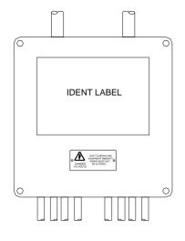
Glass-Fibre Reinforced Polyester (GRP) enclosure in light grey (RAL7000) W400mm x H405mm x D120mm with stainless steel captive crosshead screw fixed lid.
