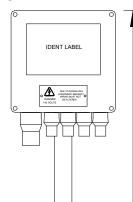
Glass-Fibre Reinforced Polyester (GRP) enclosure in light grey (RAL7000 - Squirrel Grey) W250mm x H255mm x D120mm. Lid attached with stainless steel captive crosshead screws. The product is supplied as a finished product, with an ingress protection rating of a minimum IP65 for complete assembly including glands to withstand the harsh railway environment.
